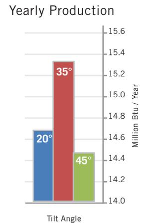
For year round hot water production, it is shown that shallower tilts produce higher annual solar fractions, though not every month in the year is higher producing. In this particular city, any production from September to March stays relatively similar between the three tilts; however, between April and August, the shallower tilts, when the most sun is available throughout the year, make the large part of yearly production.
