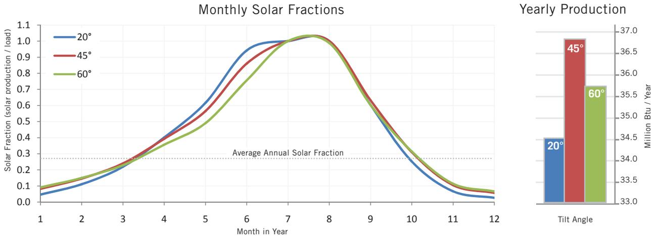
The plot above shows that a Heliodyne recommended tilt of 45° produces a higher annual solar fraction, than any other tilt. This occurs because during the time of year when space heating is necessary – February to April and August to mid October – the collectors are better positioned for solar collection when the sun is at a higher intensity.
